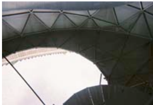
Figure 4: Primary dish, a piece of the secondary at the top, and a piece of tertiary lower right.
